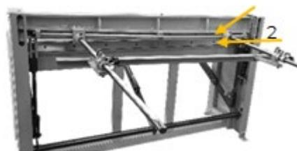
For better access to the cutting blades, remove the guide rails of the backgauge.
