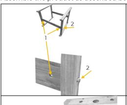
1. Place the connecting nut into the opening of the frame brace (1). Make sure that the slot of the connecting nut is aligned horizontally.
