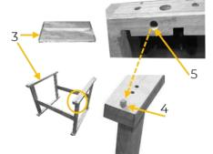
2. Place the worktop on the workbench frame (3). The wooden dowels of the workbench frame (4) should slide into the holes on the underside of the worktop (5) and fix the two parts.
